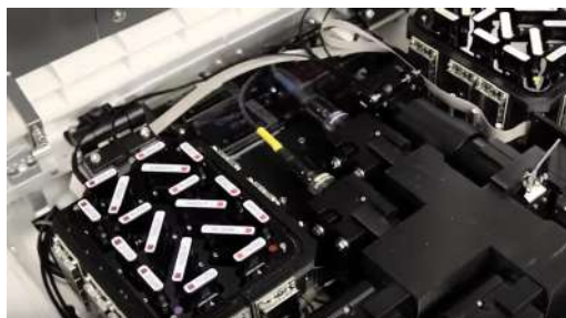
Figure 16. The optical filters in the Attune NxT Flow Cytometer are user-exchangeable, easily slotted in and out of the optical bench to maximize your capacity.
