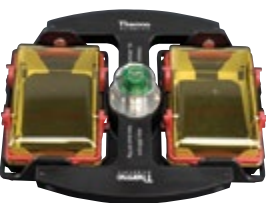
M-20 Swinging Buckets Rotor 1 , 90°, R max 127 mm
