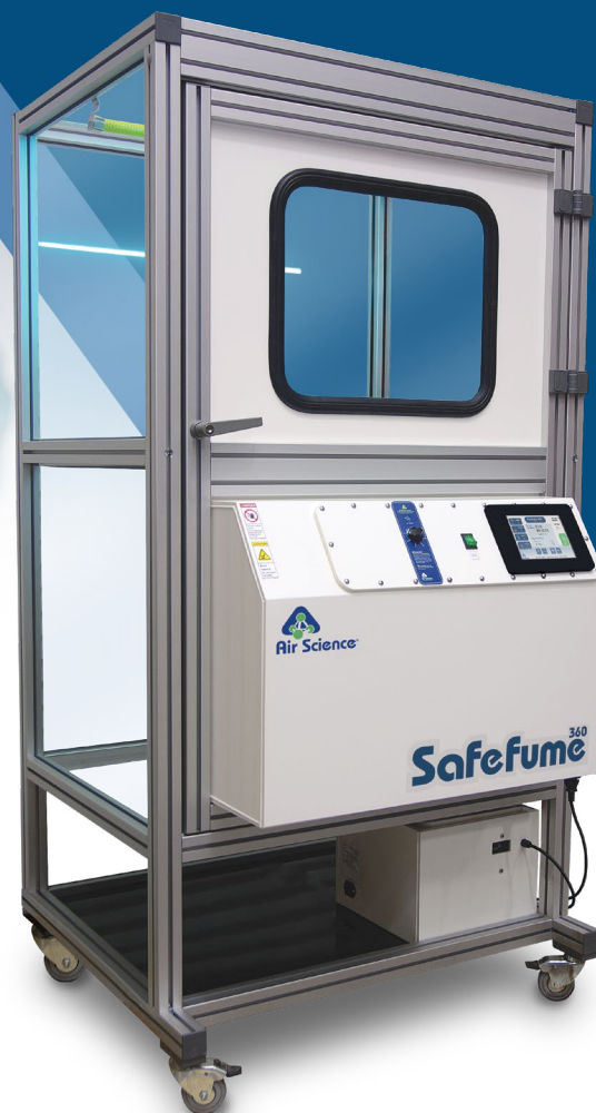
SafeFume™ 360 ARV-33T Chamber shown with optional UV Lamp and UPS
