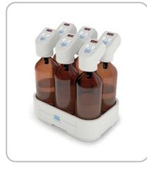
BOD Sensor System is available in 6- or 10-place configuration, including a 6- or 10-position stirring station with BOD Sensors, dark glass bottles, alkali holders for absorbing the carbon dioxide and stirring bars.
