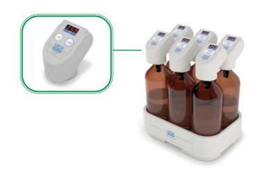
BOD EVO transfers the BOD value to the Wireless Databox<sup>™</sup> automatically.
