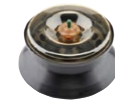
MicroClick 18 x 5 Aluminum Fixed Angle Rotor, 45°, R max 102 mm
